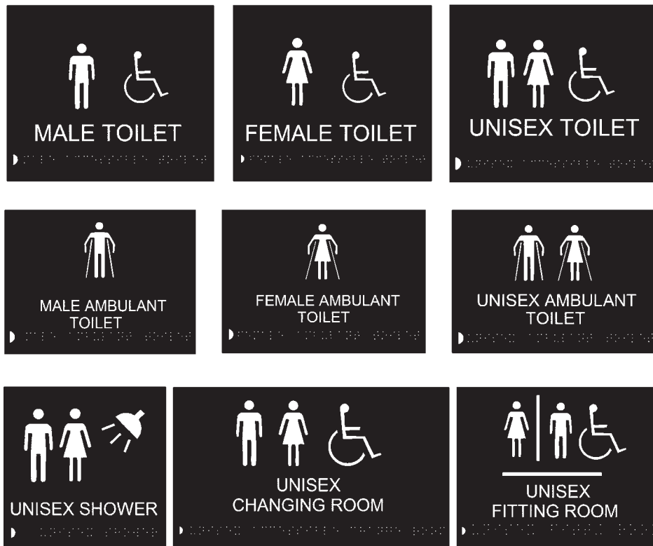
FIG. 89 SIGNAGE FOR DIFFERENT SANITARY FACILITIES
